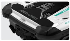
Swim Platform with Integrated LinQ System Exclusive quick-attach system on a large swim platform that allows for easy installation of accessories.
