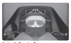
Hydraulic Steering Damper 3 steering positions to quickly control stiffness. It adds riding precision by removing undesired input in rougher conditions. It provides a premium feeling and improved control to the rider.
